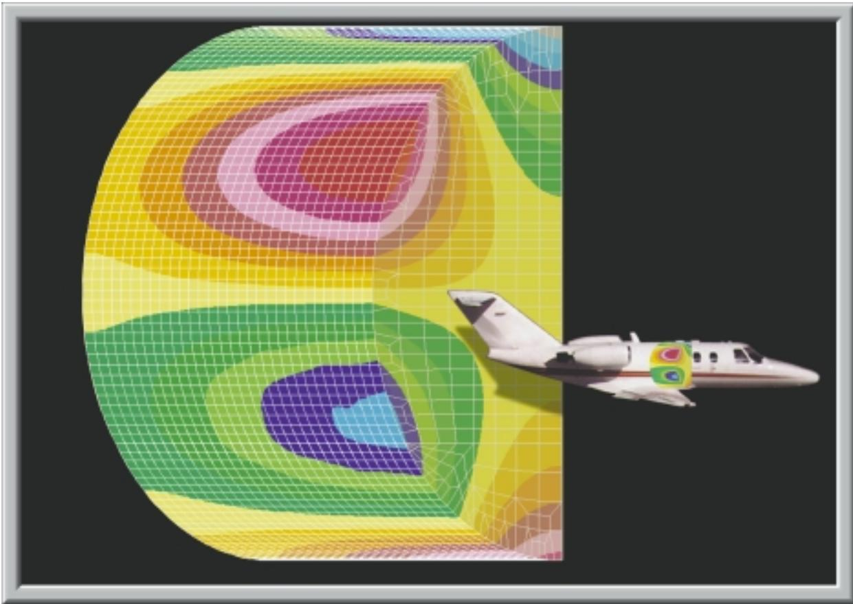
*SARA-3D was used in the analysis of a section of an aircraft fuselage model for the purpose of quieting the interior. This is the plot of the interior pressure from a point load at the top of the fuselage section. The load frequency used was 86 Hz. The resonance is a consequence of a compliant region in the fuselage, namely the windows, which happen to be near the bright red spot in the picture (The red color represents 9.8 mPa, and the lightest blue color represents -10.7 mPa.)*
