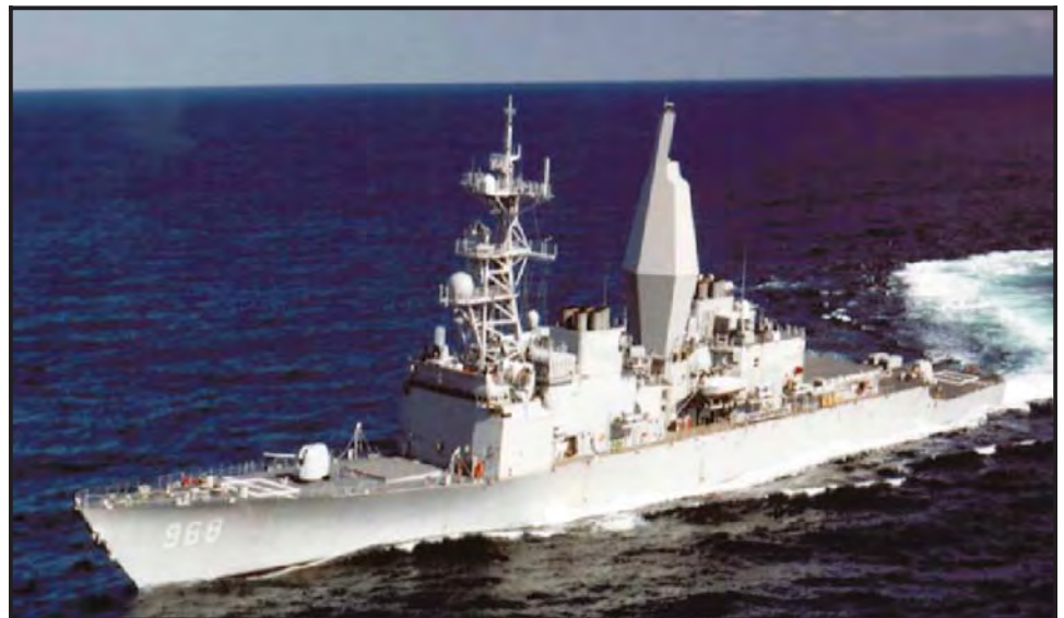
FIGURE 1. USS Radford with Advanced Enclosed Mast/Sensor (AEM/S) mast. (Courtesy U.S. Navy and SSCSD).
